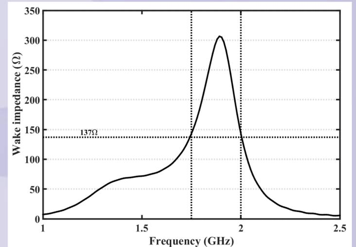
The minimum wake impedance within the operational band is 137Ω, which implies a minimum shunt impedance of ~274Ω. The peak wake impedance is 306Ω giving a peak shunt impedance of 612Ω.
