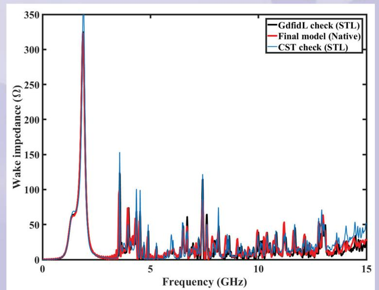
The mechanical drawings were imported into both GdfidL and CST modelling software and the results compared with those from the final design written in native GdfidL input code. The agreement was very good giving us confidence that the mechanical drawings accurately represent our requirements.
