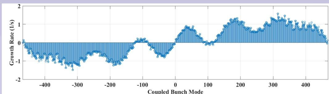
We calculated the expected growth rate of coupled bunch modes caused by the cavity, using a modified version of calculations in MatLab obtained from LNL, based on the Wang formalism.
