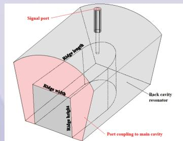
In 2017 it is planned to install some additional normal conducting cavities into the Diamond storage ring. In order to deal with the potential higher order modes in these, we are designing a longitudinal bunch-by-bunch feedback system, based on an overloaded cavity kicker, adapted to the Diamond beam pipe cross section.
