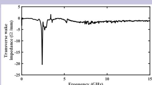
The transverse wakes were also checked and found to be a benign 20Ω/mm, which is of the same order as many other existing components.
