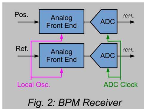
If the ADC clock is not locked/synchronized to the LLRF (beam) and the reference and position cavities are not tuned exactly to the same frequency then phase errors are introduced (since the sampling time  $T$  is not known):
