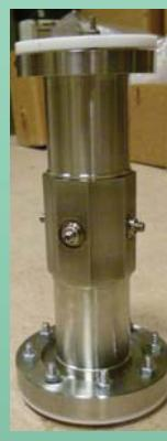
FABRICATION ERROR (GAP) ON THE LEFT ELECTRODE LEADS TO EXCENTRED ELECTRICAL CENTRE
