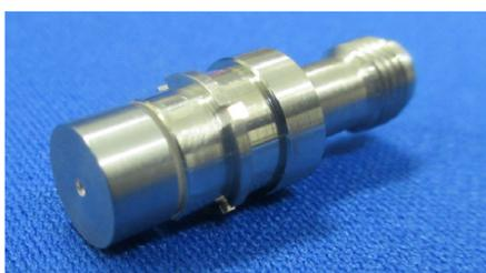
Prototype of button electrode
