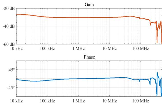
Fig. 10: Amplifier frequency response
