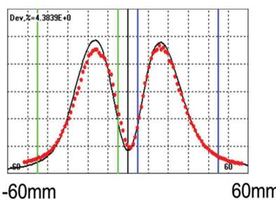
Comparison of CDR AD bunch length method with EO sampling technique
