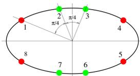
Figure 4: Eight probe points around the tube perimeter.
