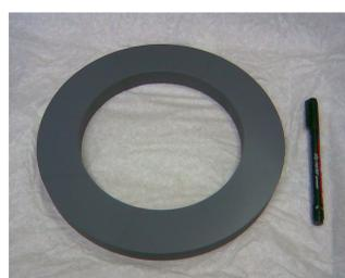
Figure 7: One of the T240/160/20-8C11 toroid cores
