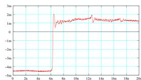
Figure 5: Step response of the final WCM output. Risettime is 60ps.
