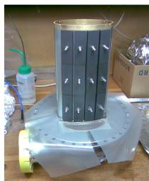
Figure 6: The inner chamber with its 4S60 absorptive tiles.
