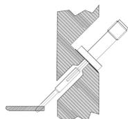
Figure 3: Detail of a feedthrough.
