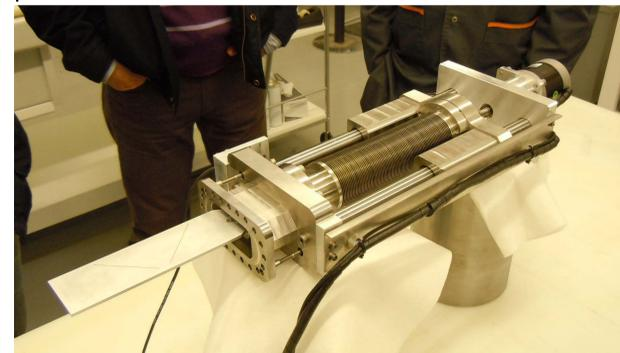
Figure 3: a scanning slit
