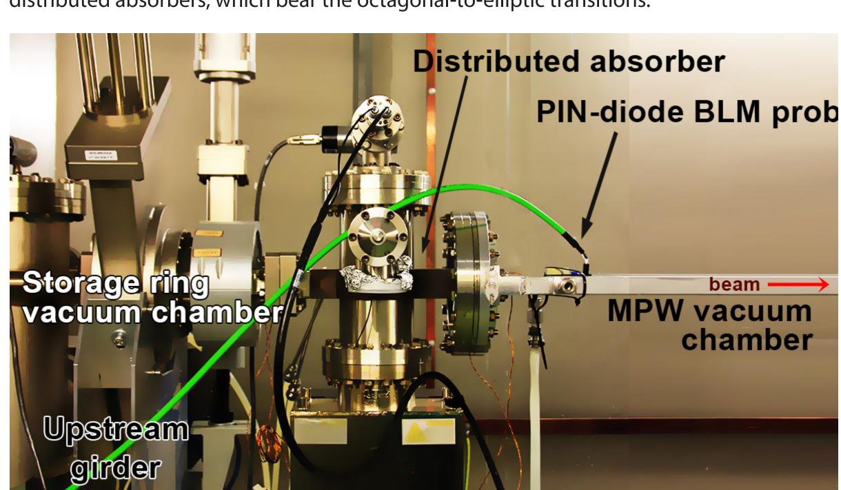
An alignment survey had indicated that the upstream girder is misaligned by 0.8mm downwards with respect to the downstream girder, thus tilting the MPW chamber. A pair of BLMs were placed on top and under the MPW chamber upstream to monitor possible beam losses. Very high, beam current-dependent losses were indeed detected, more on top of MPW than below.
