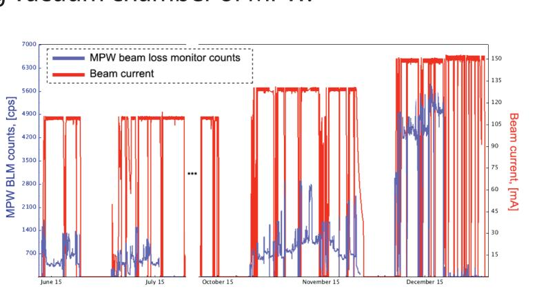
Beam losses measured on top of the MPW vacuum chamber in 2015, indicating a drastic dependence on beam current rising from 1000 cps at 120 mA to 6000 cps at 150 mA.
