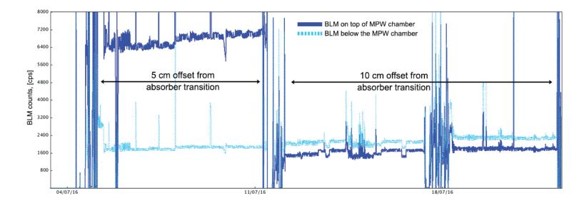
Longitudinal "scanning" of beam losses on top and bottom of the MPW vacuum chamber: the counts above decrease as the BLM gets farther from the misaligned region, while the counts below stay constant.
