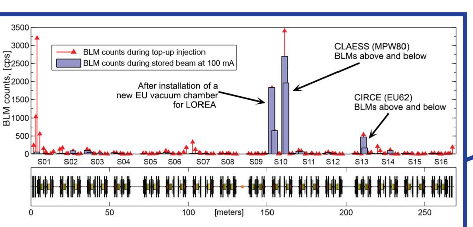
Up-to-date (02.09.2016) beam loss distribution (linear scale) around the ALBA storage ring as observed in the control room. Its shows high-loss regions, possibly related to misalignment issues in the
