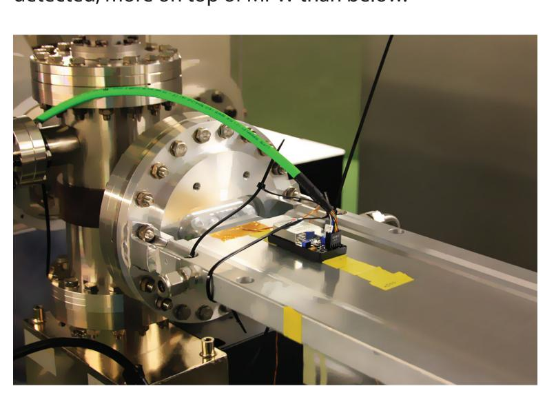
Beam loss monitor placed on top of the MPW vacuum chamber to study losses induced by misaligned storage ring sections.
