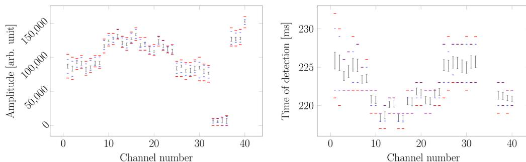
— Mean value, standard deviation — Lower and higher acceptance limits — Minima, maxima in sample
