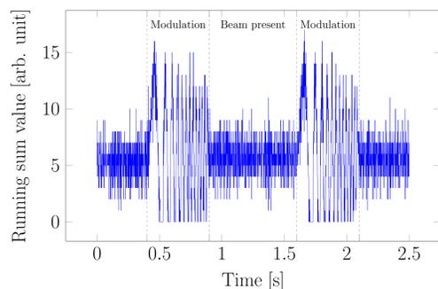
Fig. 2: Response to a 0 – 50 Hz chirp excitation in the lab.
