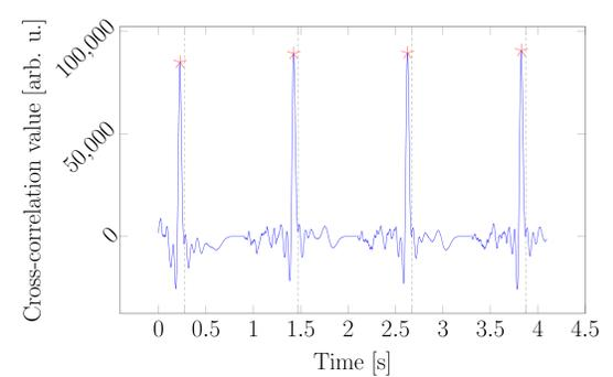
Fig. 4: Cross-correlation waveform at the PSB with a linear chirp from 0 Hz to 20 Hz.
