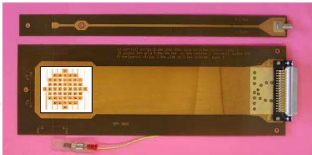
Figure 2: BPM pixel detector for beam profile with 39-pads (bottom) and single-pad (top).
