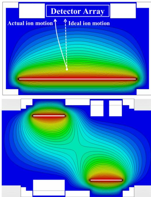
Figure 2: Non-uniform electrostatic potential distributions within the MCPM: transverse (top) and longitudinal (bottom), showing the central saddle point.
