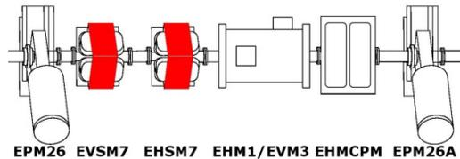
Figure 3: Schematic of the EPB1 layout surrounding the MCPM. EPM26 and EPM26A are harp monitors and EHM1/EVM3 is a dual plane position monitor.
