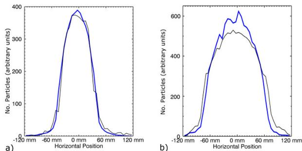
Figure 4: Comparisons of simulated (blue) and measured (black) MCPM profiles in EPB1, taken at a) low intensity operation and b) standard operating intensity.
