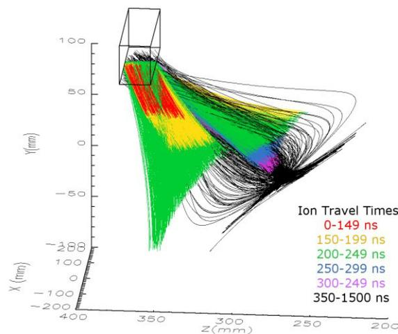
Figure 6: Trajectories of ions that reach the detectors, shown in the longitudinal plane.
