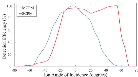
Figure 8: Variation in Channeltron detection efficiency with ion angle of incidence. The MCPM contains 4800 series Channeltrons while the SCPM uses a 4700 series.
