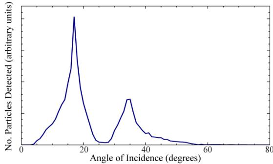
Figure 7: Longitudinal angles of incidence at which ions enter the detector.
