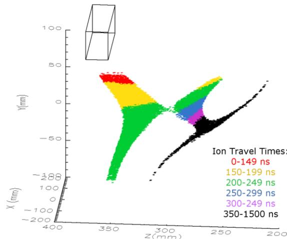
Figure 5: Initial positions of ions that travel into the detector array. The different colours denote the time of flight from creation to detection. The position of the MCPM detector array is shown as a black box.
