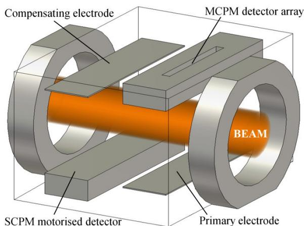
Figure 1: The layout of an ISIS profile monitor.
