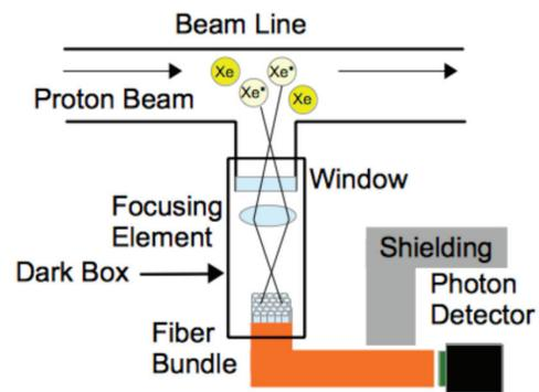
Figure 7: Light detection with optical fibers transporting light 10s of meters from the beamline to shielded MPPCs.
