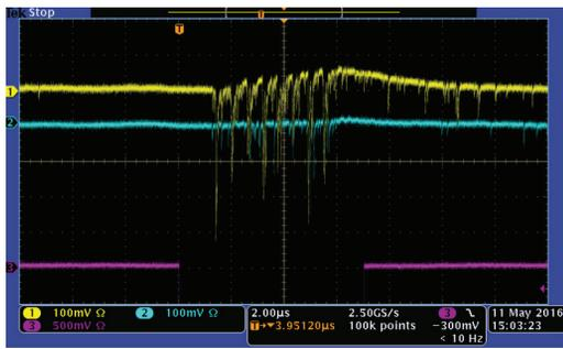
Figure 8: Noise test of silica-core optical fibers near the beamline, where the yellow curve corresponds to an unshielded fiber and the blue curve corresponds to a shielded one. Observed 8-peak noise structure corresponds to the 8-bunch J-PARC beam structure.
