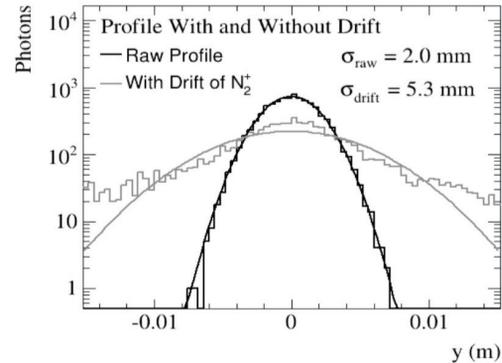
Figure 3: True beam profile and measured beam profile after drift in the beam induced space-charge field.
