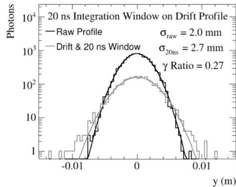
Figure 4: True beam profile and measured beam profile after drift in the beam induced space-charge field after a timing cut.
