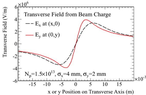
Figure 2: Transverse field induced by proton beam space-charge.
