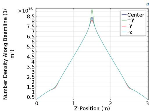
Figure 6: Number density of particles within a vacuum vessel simulated assuming steady-state gas injection by COMSOL Multiphysics®.
