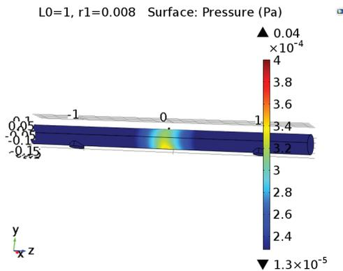
Figure 5: Pressure on the walls in a vacuum vessel simulated assuming steady-state gas injection by COMSOL Multiphysics®.
