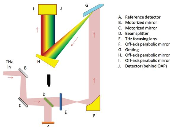
Figure 2: Preliminary broadband spectrometer design for beam length measurements. The linear polarizer is not shown.
