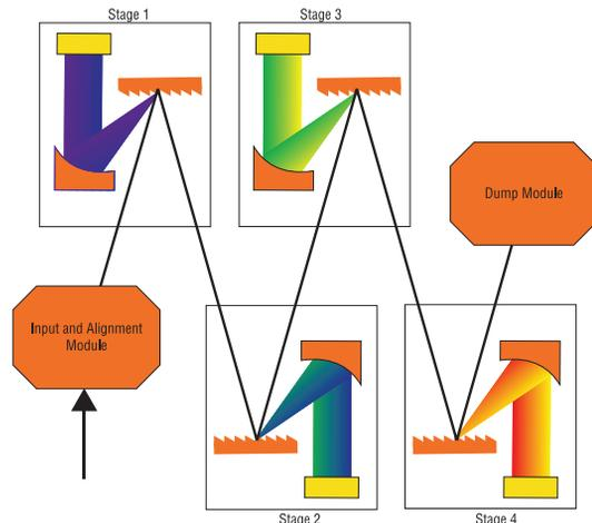
Figure 5: A cascaded spectrometer is shown with four stages, an input module, and an exit module. Additional stages can be added to expand the range of wavelengths covered or to allow smaller wavelength steps.
