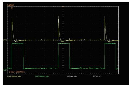
Figure 4: Response of peak detector (yellow) to a series of xenon lamp pulses (green) – right.
