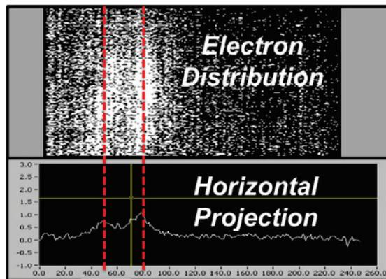
Figure 2: (top) Raw camera image showing the electron distribution intensity. (bottom) Projection of the distribution onto the horizontal axis.
