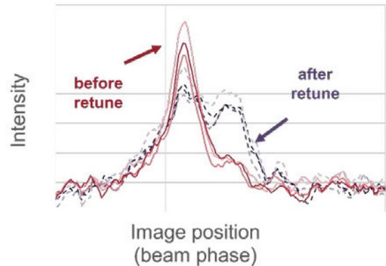
Figure 5: Bunch changes after tuning higher current.
