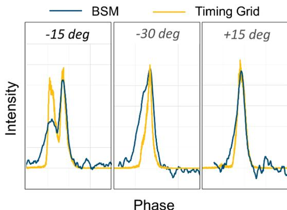
Figure 6: Bunch shapes measured by BSM and timing grid under three different bunching conditions (ReA cavity phases -15, -30, and +15 degrees).
