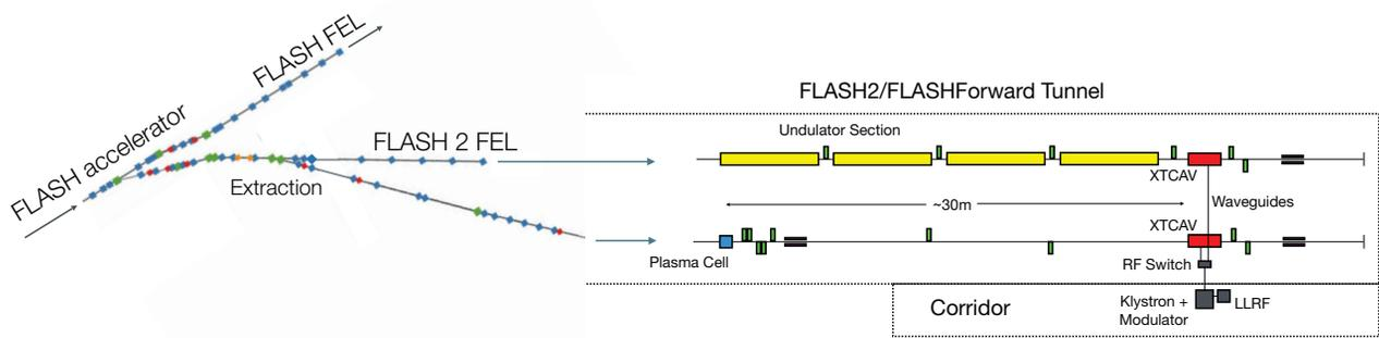
Figure 1: A schematic of the FLASH beam line, demonstrating extraction into FLASH2, with subsequent extracting into FLASHForward. A sketch of the proposed experimental hall layout is also shown, with the placement of the shared RF source and respective deflecting cavities illustrated.
