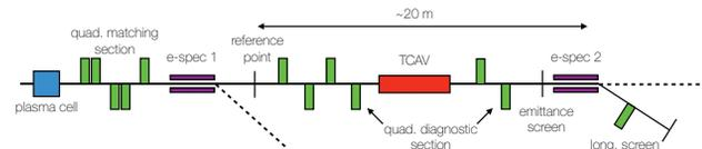
Figure 2: A sketch of the post-plasma cell beam line optics configuration defined by the constraints outlined in Tab. 2.
