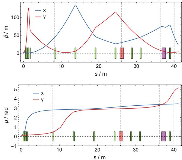
Figure 5: The beta function and phase advance in both transverse planes for the matched longitudinal phase space case. As in Fig. 3, the optics elements and screens are illustrated on each plot.
