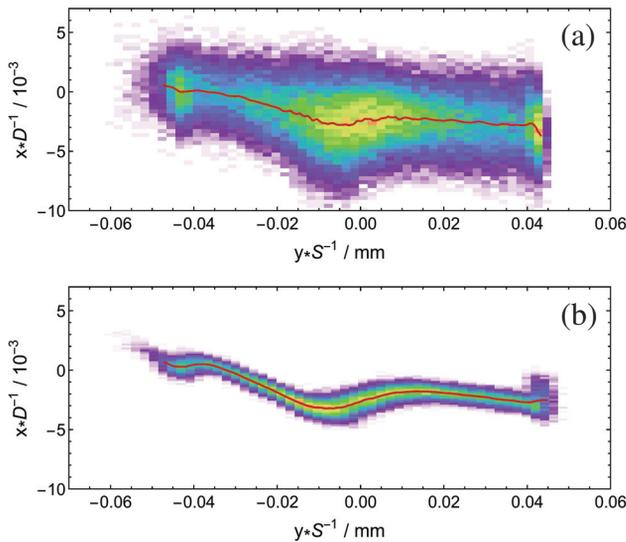
Figure 7: The reconstructed longitudinal phase space at the dispersive screen for a streaking voltage of a) 30 MV, and b) 6 MV.
