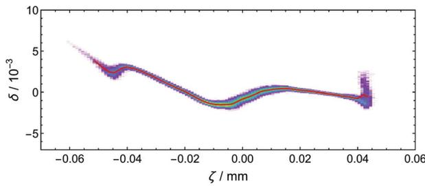
Figure 6: The longitudinal phase space of the input distribution, used for particle tracking in the FLASHForward eLlegant beam line. The  $y$ - and  $x$ -axis represent the relative energy spread and centre of mass frame of the bunch, respectively.
