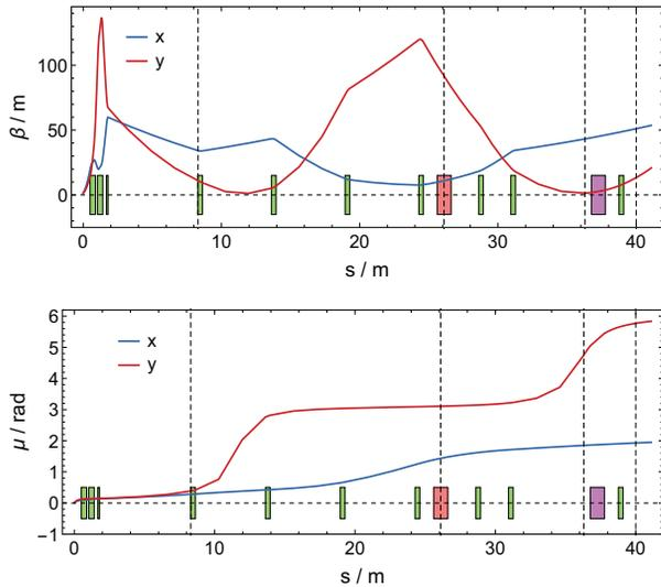
Figure 3: The beta function and phase advance in both transverse planes for the matched slice emittance midpoint case. The location of the quadrupoles (green), TDS (red), and dipole (purple) are indicated on the plot. The vertical dashed lines represent (from left to right) the reference point, centre of the TDS, emittance screen, and dispersive screen.
