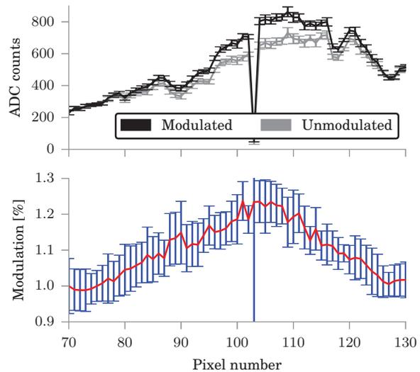
Figure 2: Top: modulated and un-modulated (averaged) signals recorded with KALYPSO. Bottom: relative modulation of the laser pulse (single-shot). In both plots the error bars show the standard deviation.
