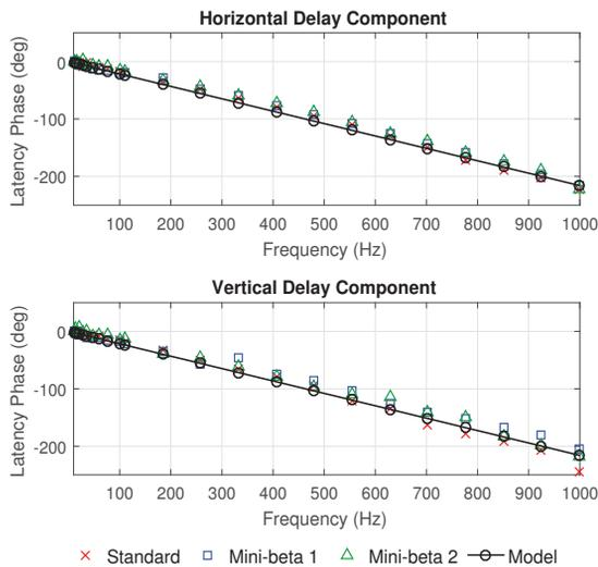
Figure 3: Phase introduced by the system latency in horizontal and vertical planes for a standard corrector (red ‘x’) and mini-beta correctors (blue ‘□’ and green ‘Δ’) compared with a linear fit (black ‘o’) of a 600  $\mu$ s delay.
