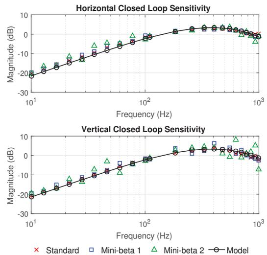
Figure 4: Measured sensitivity in horizontal and vertical planes for a standard corrector (red ‘x’) and mini-beta correctors (blue ‘□’ and green ‘Δ’) compared to the theoretical response (black ‘o’).
