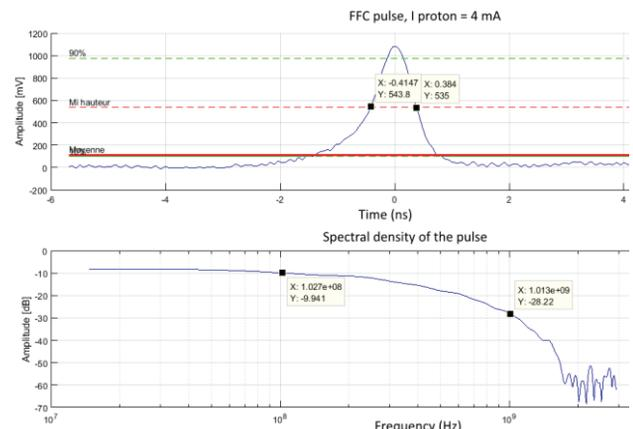
Figure 9: Spectral density of the proton pulse.
