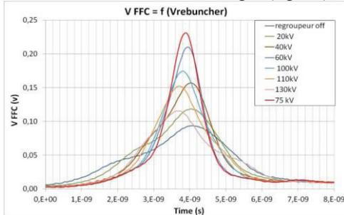
Figure 10: FFC pulse in function of the rebuncher voltage.
