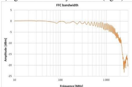
Figure 7: FFC frequency spectrum
