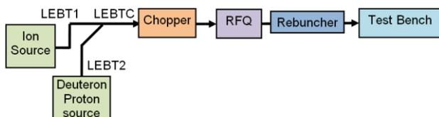
Figure 1: Injector diagram.
