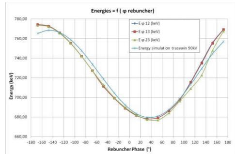
Figure 4: Energy in function of the rebuncher phase.
