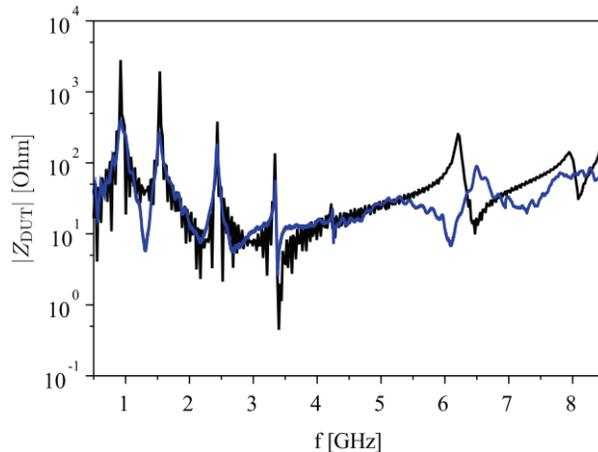
Figure 6:  $Z_{DUT}$  obtained by measurement (blue) and by simulation for  $\epsilon_r = 10.7$  (black).
