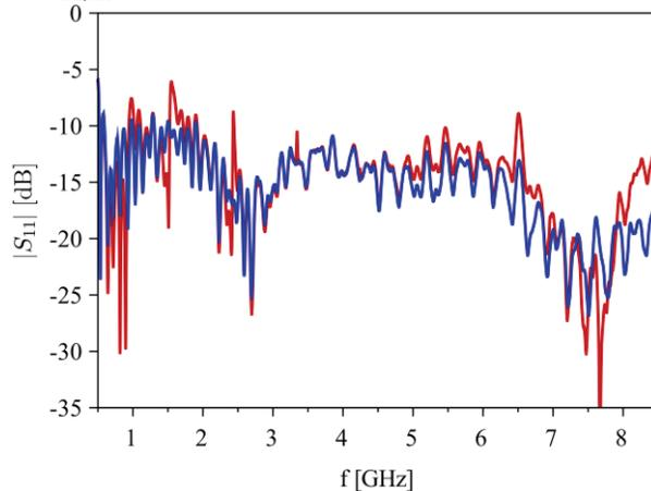
Figure 5: Measured reflection coefficients  $S_{11,ref}$  (blue) and  $S_{11,all}$  (red).
