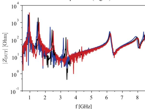
Figure 4: Simulated  $Z_{DUT}$  using  $\epsilon_r = 9.9$  (red),  $\epsilon_r = 10.7$  (black) and  $\epsilon_r = 12.0$  (blue).
