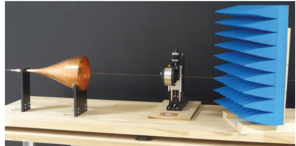
Figure 3: Goubau Line used for reflection measurements. The DUT is supported by micro-movers, allowing accurate positioning.
