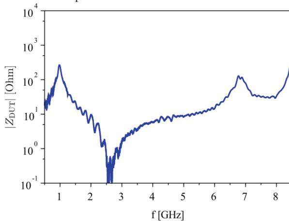
Figure 7: Measured coupling impedance for a centered DUT.
