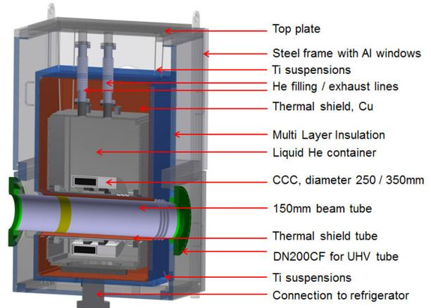
Figure 6: Schematic view of the FAIR CCC cryostat.
