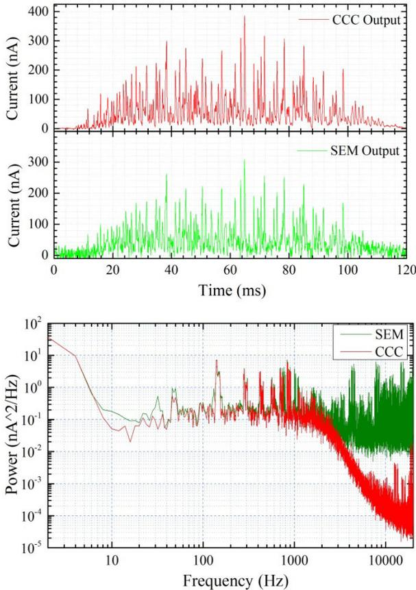
Figure 2: Upper: Comparison of the beam current signal measured by CCC and SEM. Lower: Corresponding FFT spectrum with normalized intensities and averaged over 9 spills.
