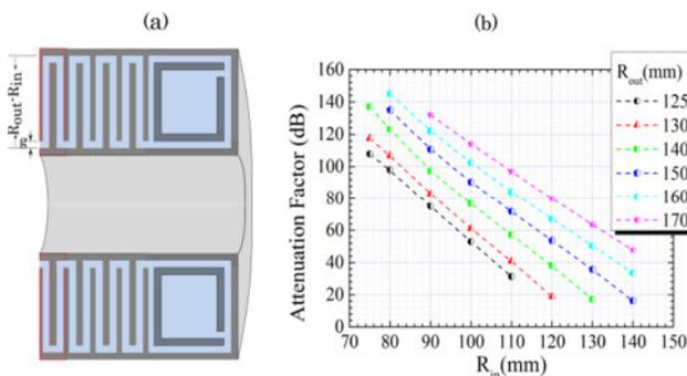
Figure 5: (a) Cross-sectional view of the magnetic shield geometry model. (b) Attenuation factor plotted for various inner and outer diameters of the magnetic shield.
