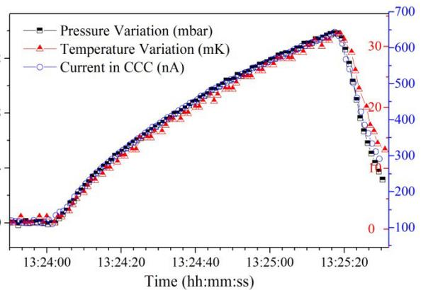
Figure 4: Time development of CCC output at variation of pressure and temperature.
