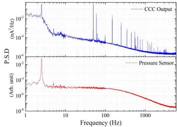
Figure 3: FFT of the output signals of CCC and pressure sensor showing the influence of pressure variation.
