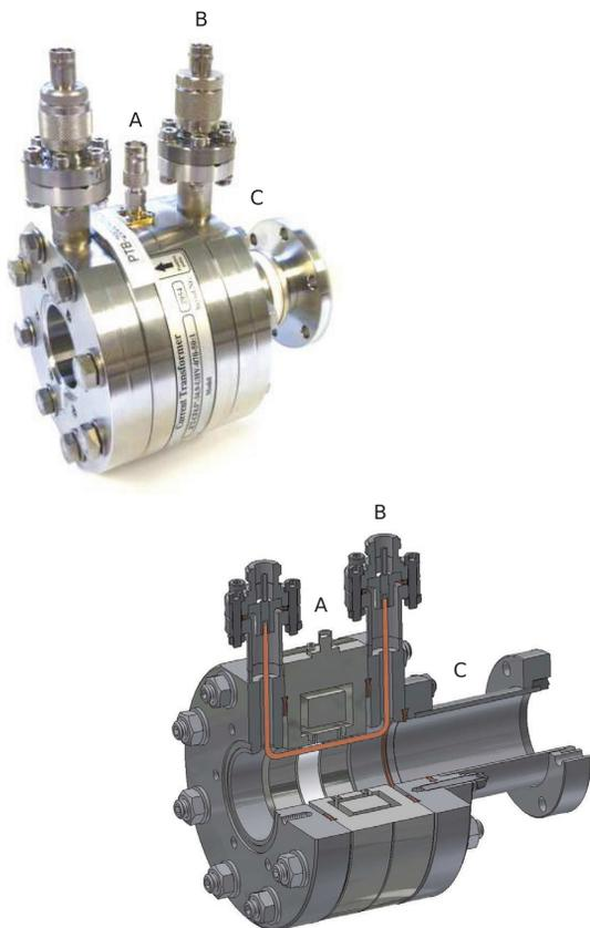
Figure 2: Photo (top) and sectional drawing (bottom) of the ICT (A) with an in situ wire (Q-loop) through the ICT screwed on electrical feedthroughs at additional flanges (B) and a vacuum ceramic break (C).
