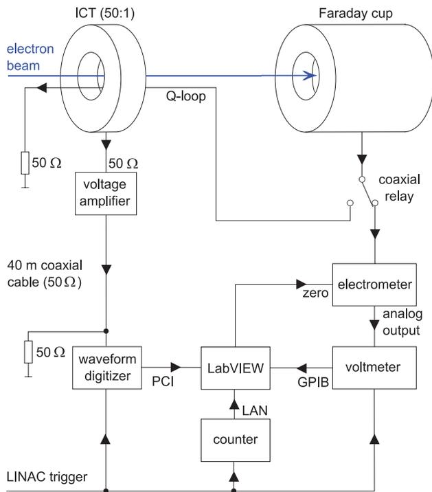
Figure 5: Block diagram of the setup.
