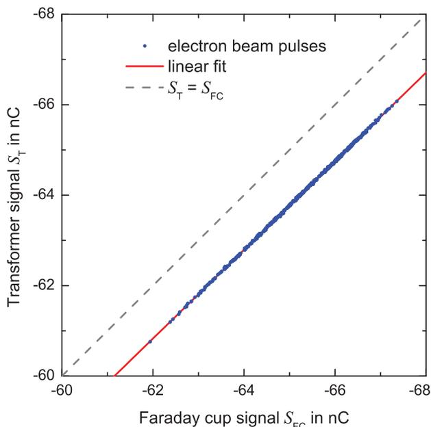
Figure 7: Transformer signal  $S_T$  of 500 sequent single beam pulses as a function of the simultaneously collected corresponding charge  $S_{FC}$  from the FC.
