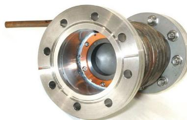
Figure 3: Photo of the Faraday cup glued into a vacuum adapter with a water cooling coil welded on the outside wall.
