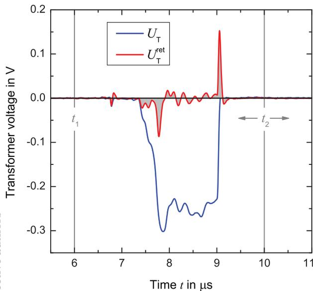
Figure 6: Blue curve: time resolved transformer voltage  $U_T(t)$  for a typical LINAC beam pulse (27 MeV,  $-60$  nC). Red curve: transformer voltage at return of the FC current through the ICT via the Q-loop  $U_T^{\text{ret}}(t)$ . Pulse integration limits:  $t_1 = 6 \mu\text{s}$  and  $t_2 \geq 9.3 \mu\text{s}$ .
