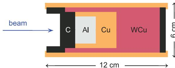
Figure 4: Drawing of the structure of the Faraday cup.
