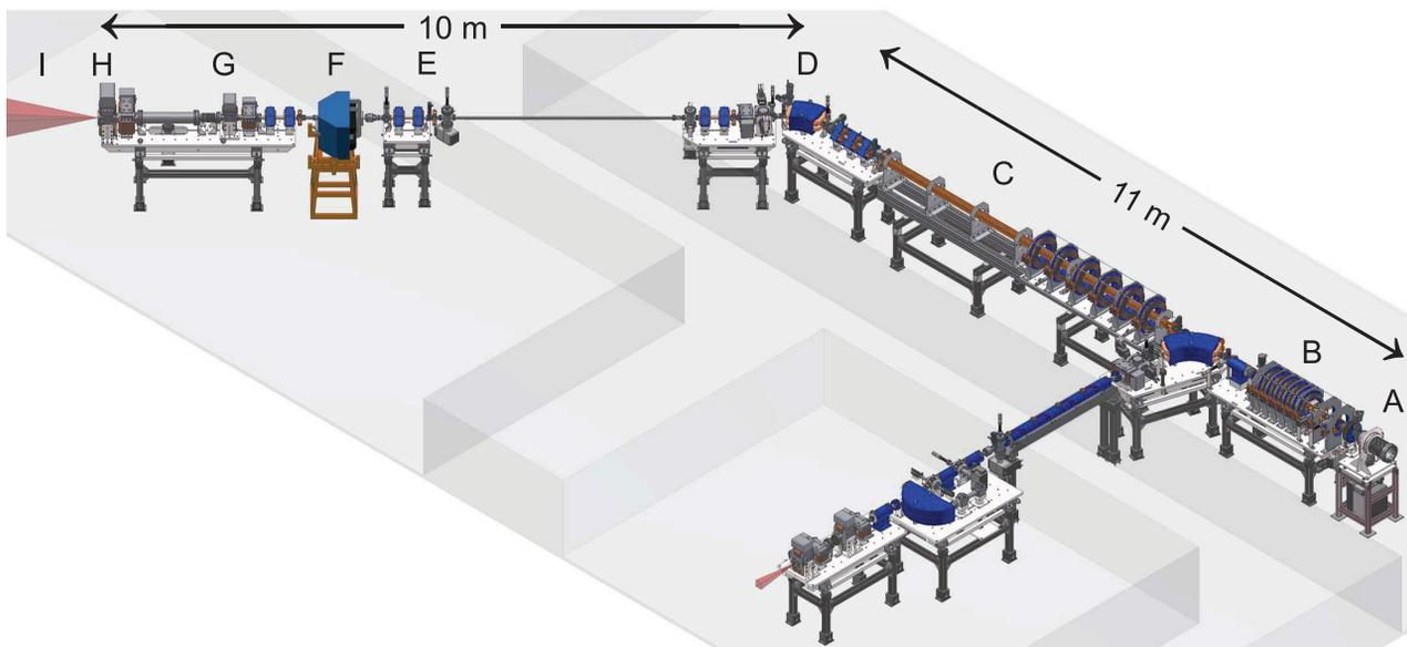
Figure 1: Drawing of PTB's electron LINAC for fundamental research in dosimetry for radiation therapy. A: electron gun. B: low-energy section (0.5 to 10 MeV). C: high-energy section (6 to 50 MeV). D: dipole magnet for energy separation and beam dump. E: collimator. F: magnetic spectrometer. G: ICT. H: Faraday cup or metal target. I: photon radiation. Gray areas: walls of the radiation protection bunker.
