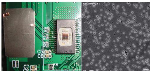
Figure 3: Polymer track detector and the DUT. SEM micrograph of polymer track detector.
