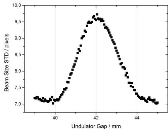
Figure 4: Undulator gap scan versus heating of the electron bunches by displaying bunch width standard deviation in pixels.
