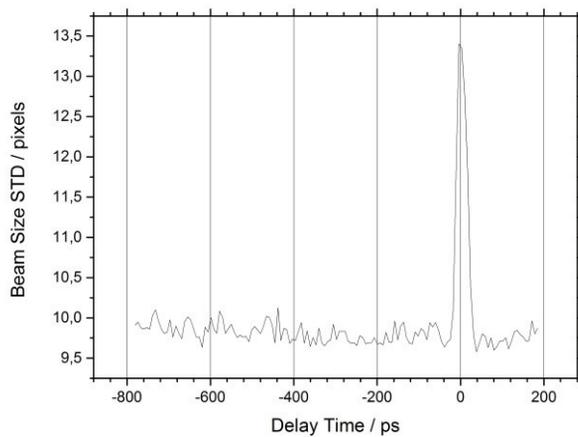
Figure 2: Fine delay line scan illustrating the first sign of heating of the electron bunches by displaying bunch width standard deviation at the dispersive section vs delay line position given in ps.
