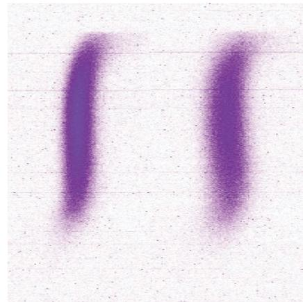
Figure 3: OTR screen in dispersive section after the laser heater and TDS switched on with left, only laser blocked, right, laser unblocked clearly showing a fuzzier trace.
