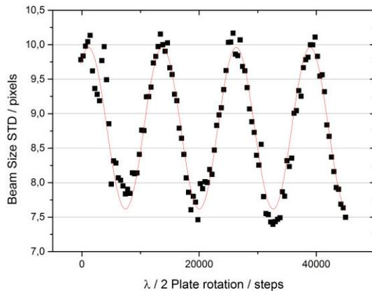
Figure 6: Laser energy scan by rotating  $\lambda/2$  plate before polarization dependant beam splitter cube.
