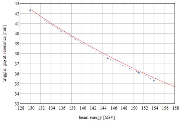
Figure 5: Measured and theoretical undulator / wiggler gap vs. beam energy.
