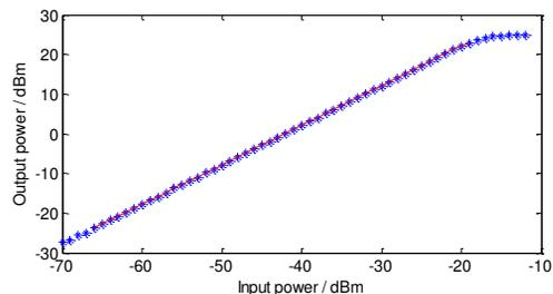
Figure 7: Gain line test of the RF front end.
