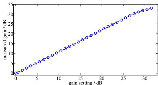
Figure 9: Gain line test result of the DBPM prototype.
