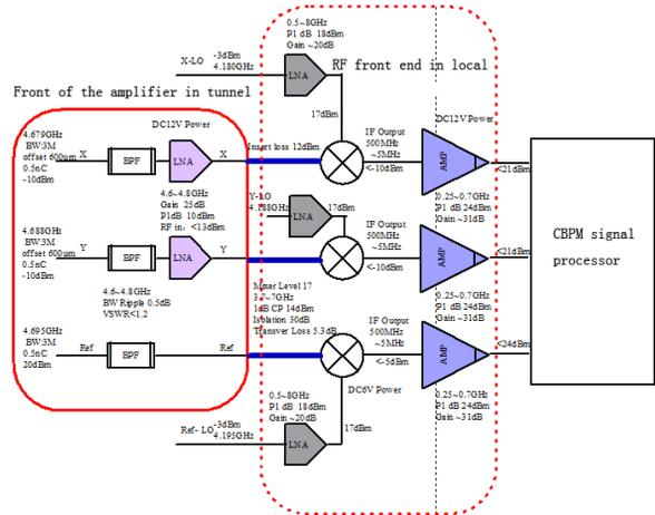
Figure 5: Block diagram of the RF front end.
