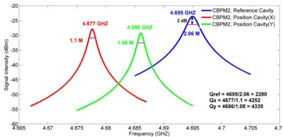
Figure 4: S21 parameter of the CBPM2 measured by network analyzer.
