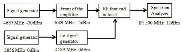
Figure 6: Diagram of the RF front end test in laboratory.
