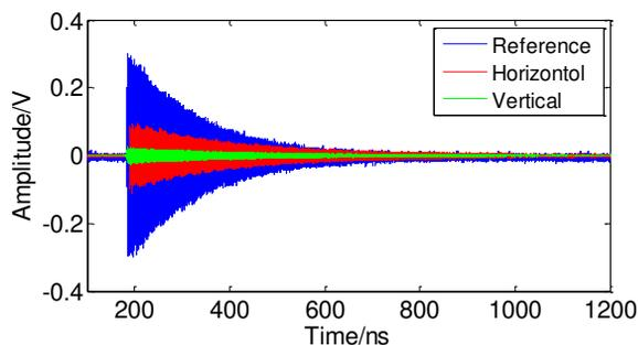
Figure 12: RF signals of the CBPM.
