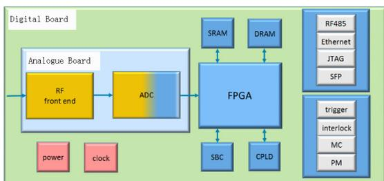
Figure 8: Simplified diagram of the DBPM processor.
