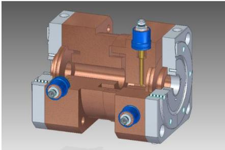
Figure 3: Three-dimension structure of the high Q CBPM.
