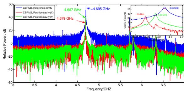
Figure 13: Frequency spectrum of the CBPM.
