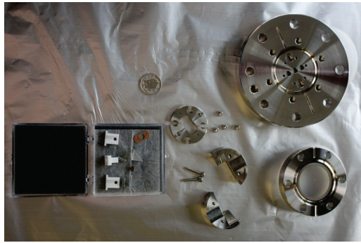
Figure 3: Pick-up components: ceramic holders, prisms and crystal.
