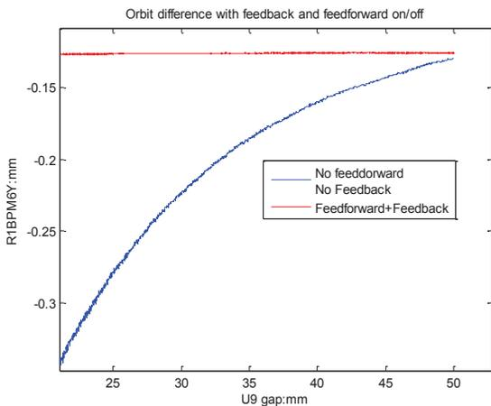
Figure 6: U9 gap control and orbit perturbation with feedback and feedforward on/off. Blue line is no feedback, no feed forward. Red line is feedback and feed forward on.
