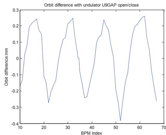
Figure 4: Full orbit difference between U9 gap open and close without orbit feedback and feed forward control.
