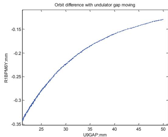
Figure 3: U9 gap moving without orbit feedback. There is 200um orbit perturbation in the RIBPM6Y.
