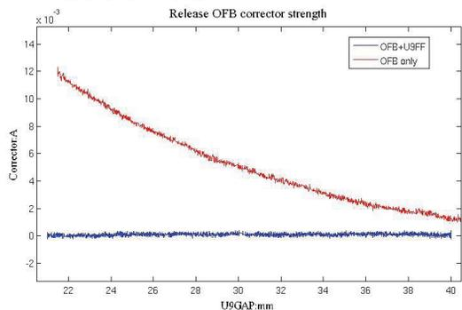
Figure 5: Corrector power-supply reading when U9 gap control with feed forward or feedback system.
