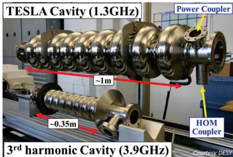
Figure 1: Picture of a TESLA and a 3<sup>rd</sup> harmonic cavity.
