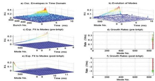
Figure 4. Grow/damp experiment of horizontal plane at beam current 300 mA with five in-vacuum IDs close gap. Resistive wall and ion induced instabilities are dominated. Feedback gain is set at minimum. Increase damping rate is easily by increase gain of the feedback loop.
