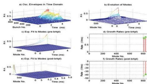
Figure 9: Grow/damp experiment of vertical plane at beam current 400 mA.
