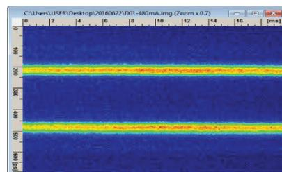
Figure 11: Longitudinal stable beam observed at 480 mA on June 22, 2016.
