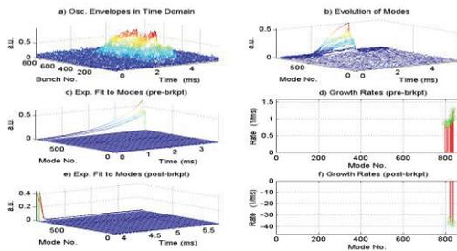
Figure 8: Grow/damp experiment of vertical plane at beam current 360 mA.
