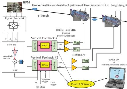
Figure 3: Configuration of the vertical bunch-by-bunch feedback loops.
