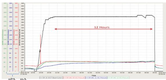
Figure 13: Vacuum pressure increase two times compare to 30 mA observed by the downstream ion gauge of horizontal kicker and vertical kicker #1 for 12 hours 400 mA operation from 21:00, September 6 to 09:00, September 7.
