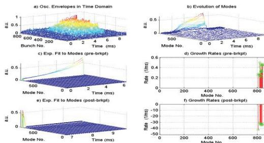
Figure 7: Grow/damp experiment of vertical plane at beam current 300 mA with five in-vacuum IDs close gap.
