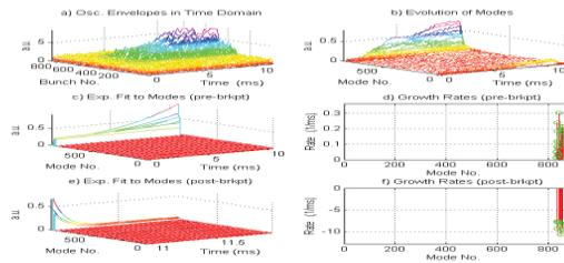
Figure 6: Grow/damp experiment of vertical plane at beam current 93 mA.
