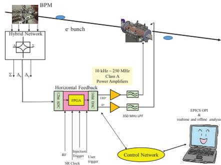
Figure 2: Configuration of the horizontal bunch-by-bunch feedback loop.
