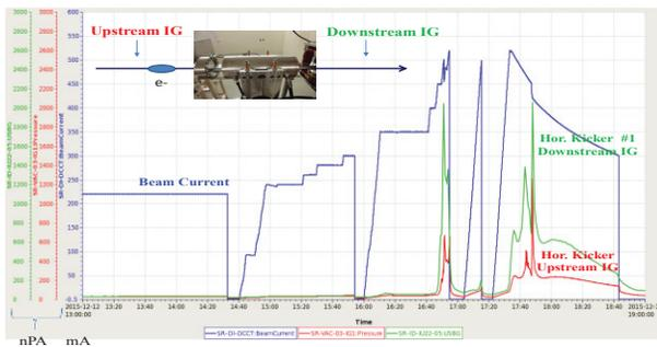
Figure 12: Vacuum burst happened when stored beam current over certain threshold (450 mA~ 520 mA) for a short duration on December 12, 2015. Ion gauge near downstream of horizontal stripline kicker detect a huge pressure spike which caused sudden reduce of beam current.
