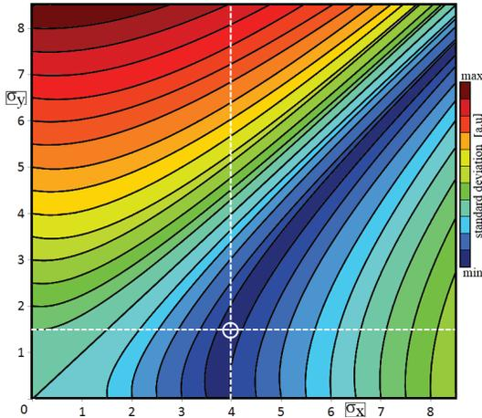
Figure 6: 2D plot of position standard deviation vs. beam size. For beam with dimension  $\sigma_x = 4$  mm,  $\sigma_y = 1.5$  mm.
