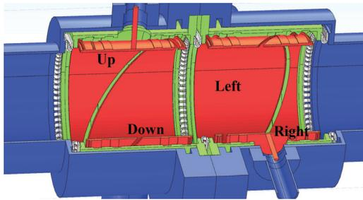
Figure 2: Cut view on diagonally cut BPM model, red: electrodes, green: grounded housing, blue: beam pipe.
