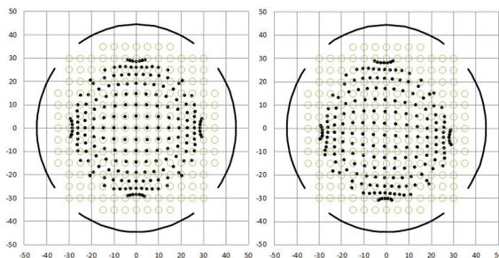
Figure 4: Projection plot of ideal and misaligned strip type BPM.
