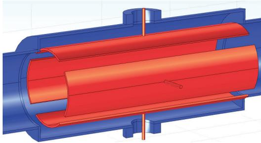
Figure 3: Model image of simplified strip type BPM, red; electrodes, blue; beam pipe.
