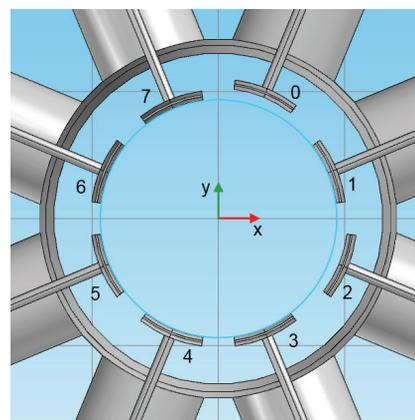
Figure 5: Cross-sectional view on eight strip BPM.
