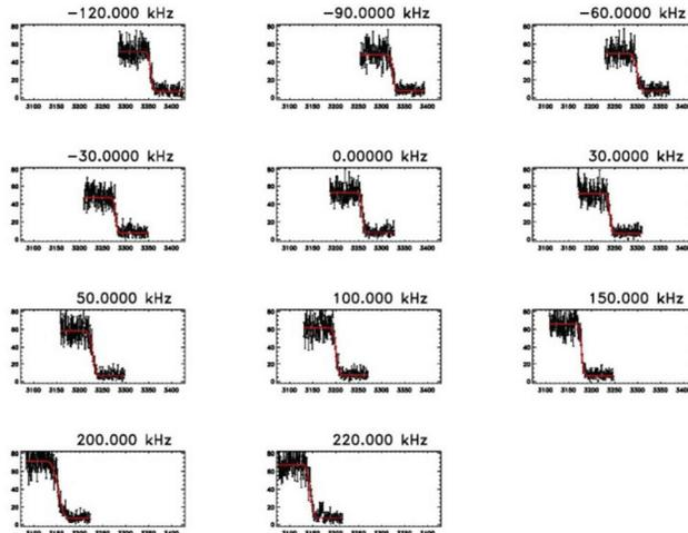
Figure 3: Example for a measurement for general storage ring diagnostics: the radio frequency was shifted and the shift in electron energy was observed by Compton backscattering (x-axis: HPGe detector channel, y-axis: counts).
