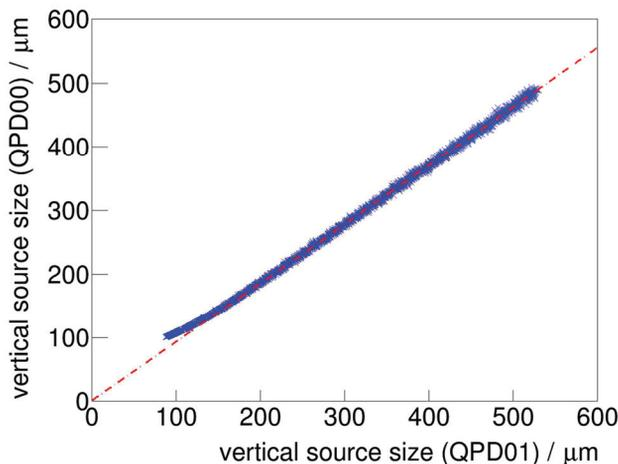
Figure 6: Measured vertical beam size by the two optical imaging systems.
