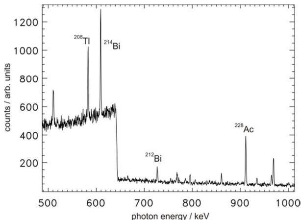
Figure 2: Typical spectrum of back-scattered photons recorded with an HPGe detector, here at 600 MeV electron beam energy. Lines from suitable radio-nuclides used for the energy calibration of the HPGe detector are also shown.
