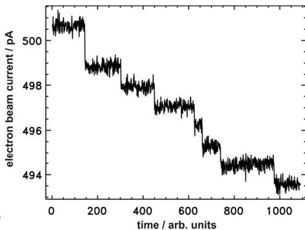
Figure 4: Electron beam current measurement by electron counting for an electron energy of 540 MeV.
