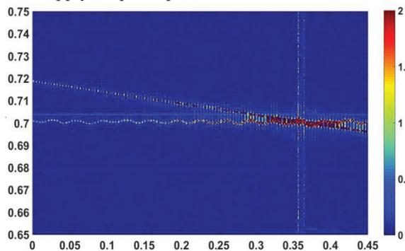
Figure 11: Measurement of the vertical betatron tune with FPM.
