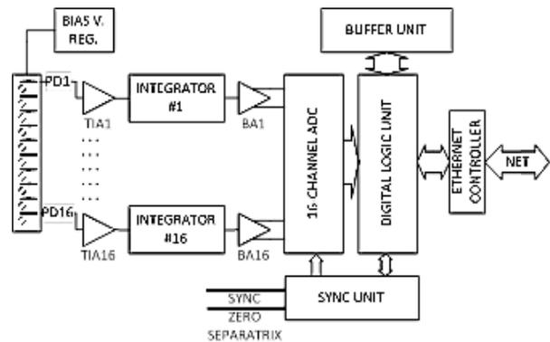
Figure 5: Functional diagram of the device.
