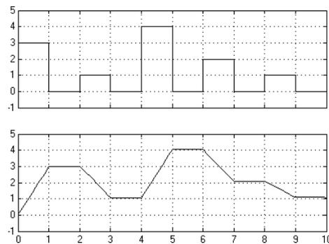
Figure 6: The integrator model in Simulink. Input signal (the 1st diagram) and output signal (the 2nd diagram).
