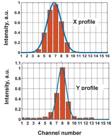
Figure 8: The vertical and radial beam profiles of a single bunch acquired with APDA at a single beam turn.
