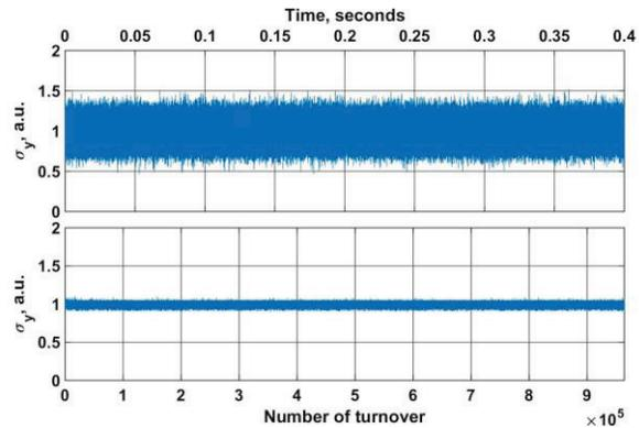
Figure 9: Comparison of an accuracy of the old (upper plot) and the new (lower plot) versions of FPM.
