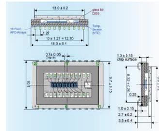
Figure 4: Package of AA16-0.13-9 APD linear array.
