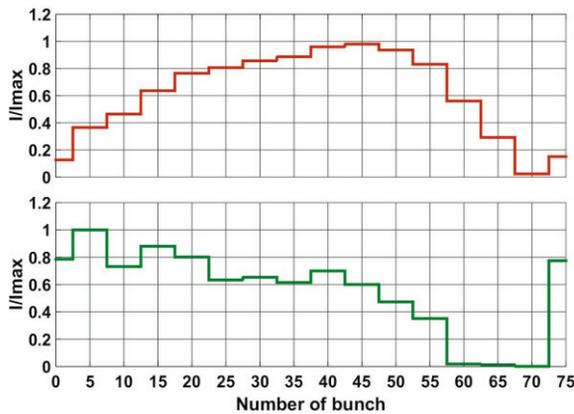
Figure 7: The integrated signal from the channel of APDA recorded by ADC.
