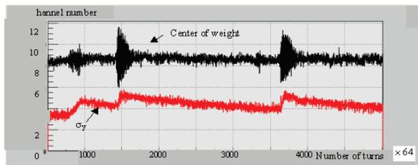
Figure 3: Beam dipole oscillations (black plot) and  $\sigma_y$  behavior (red plot) during the beams convergence at the interaction point. Duration of the single turn is 1220 ns. The channel constant is 0.12 mm.
