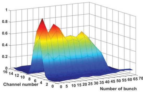
Figure 10: Vertical profiles of the bunches recorded at one beam turn.
