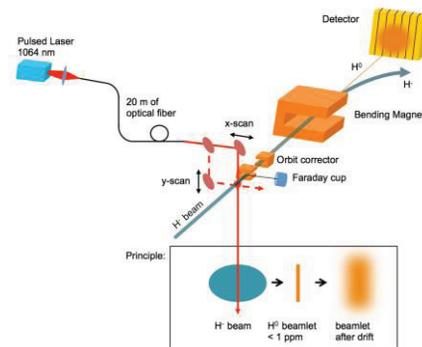
Figure 4: The laser emittance meter at CERN's Linac4.
