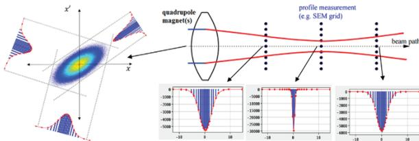
Figure 3: Using tomography to reconstruct the initial phase space distribution in a linac or transport line.
