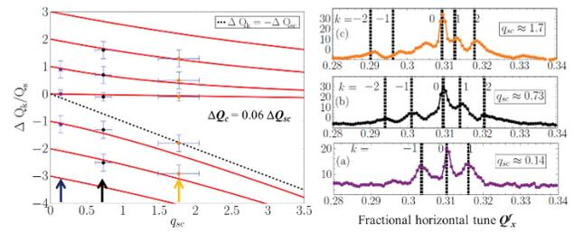
Figure 7: Simulated and measured synchrotron sideband separation for various space charge regimes at the GSI SIS18 (left). Corresponding tune spectra (right).
