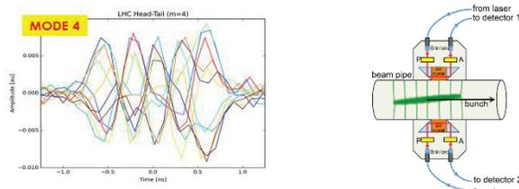
Figure 8: A mode 4 head-tail instability captured on a single bunch in the LHC using direct sampling (left). Schematic representation of an electro-optical BPM (right).
