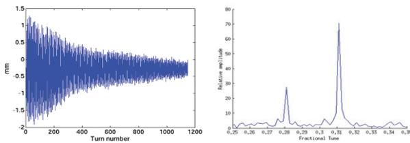
Figure 5: BPM response to a beam excited with a kick (left). Frequency spectrum in the presence of coupling (right).
