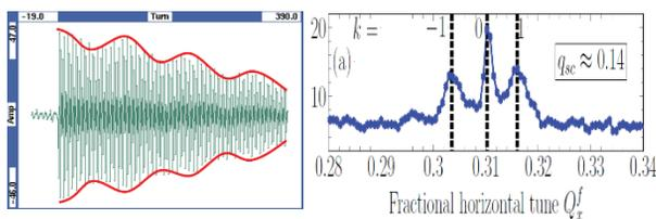
Figure 6: Amplitude modulation of the BPM response in the presence of synchrotron motion and chromaticity (left). Frequency spectrum (right).
