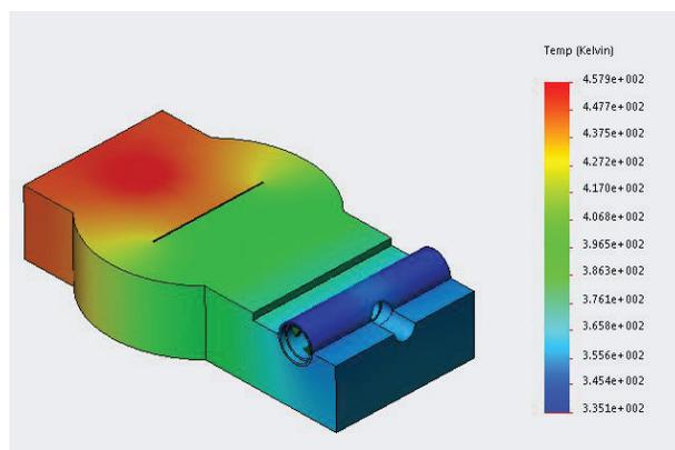
Figure 2: IPF slit model with thermal analysis.
