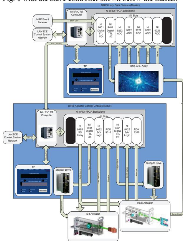
Figure 6: Emittance control system hardware diagram.
