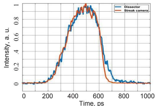
Figure 4: Comparison of the beam profiles acquired by the dissector and streak camera,  $I_b \approx 12 \text{ mA}$ .
