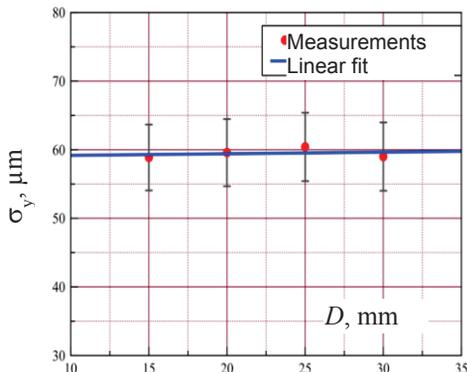
Figure 2: Vertical beam size determined with a different slit separation  $D$ .
