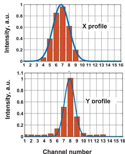
Figure 8: The vertical and radial beam profiles of a single bunch acquired with APD at a single beam turn.
