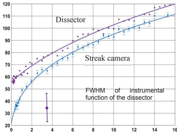
Figure 6: Beam length vs beam current measured by optical dissector and streak camera at  $E = 446$  MeV.
