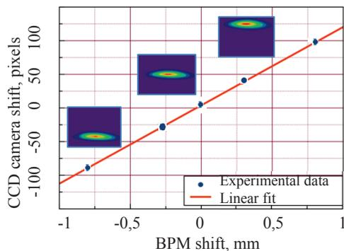
Figure 3: Shift of the beam image at the CCD camera vs BPM data.
