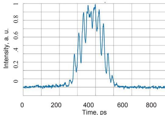
Figure 5: Distortions of the signal of the dissector caused by synchrotron oscillations,  $I_b \approx 2 \text{ mA}$ .
