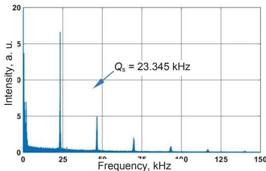
Figure 7: Synchrotron frequency obtained by Fourier transform of the dissector signal
