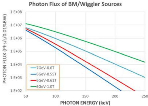
Figure 2: Spectral photon flux through a 10  $\mu\text{m}$  square pinhole at 8.5 m from an APS-U bend magnet/wiggler source with 6-GeV/200 mA electron beam. Pinhole flux of current APS source (7GeV/100mA) is shown for comparison.
