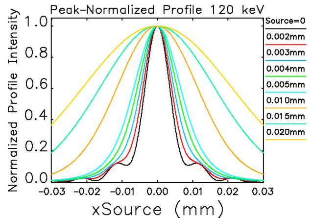
Figure 1: Fresnel diffraction profile using monochromatic 120 keV photons for zero source size; and convolution with Gaussian source with rms width of 2 – 20  $\mu\text{m}$ . All profiles are normalized at the peak for easy comparison.
