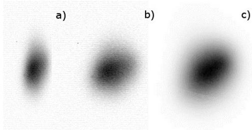
Figure 4: Raw OTR image (a), OTR image transformed to the beam coordinate space (b), YAG image (c). Beam energy is 300 keV.
