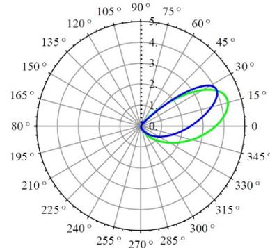
Figure 1: OTR intensity emitted at 90° to the beam direction as function of the angle  $\psi$  for beam energies 100 keV (green) and 300 keV (blue). Data plotted by the green line were multiplied by a factor of 3.
