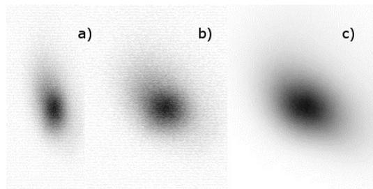
Figure 6: Raw OTR image (a), OTR image transformed to the beam coordinate space (b), YAG image (c). Beam energy is 100 keV.
