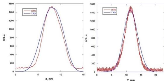
Figure 5: Horizontal and vertical beam profiles obtained from OTR and YAG images. Beam energy is 300 keV.
