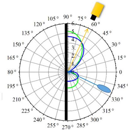
Figure 2: OTR intensity from a target tilted by an angle  $\psi = 25^\circ$  as function of the observation angle  $\theta$  for beam energies 100 keV (green) and 300 keV (blue). Data plotted by the green line were multiplied by a factor of 3. Vertical black line indicates orientation of the OTR target.
