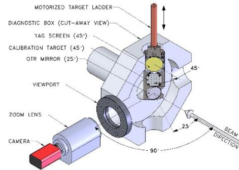
Figure 3: The experimental setup for OTR low energy imaging.
