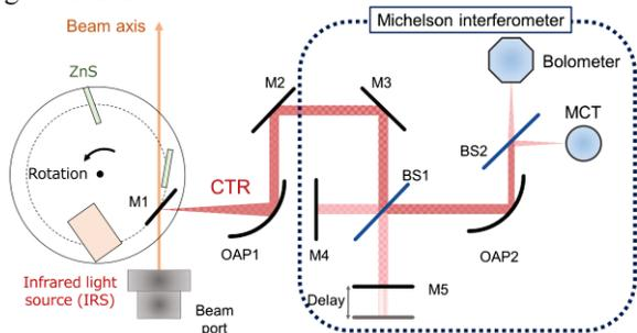
Figure 2: Schematic diagram of the Michelson interferometer. M: aluminium mirror, OAP: off-axis parabolic mirror, BS: beam splitter, MCT: Mercury cadmium telluride detector.
