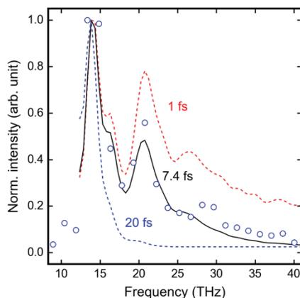
Figure 5: Frequency spectrum of CTR. The solid line denote the fitting curve based on sensitivity model. The red and blue dashed lines denote curves calculated based on sensitivity models.
