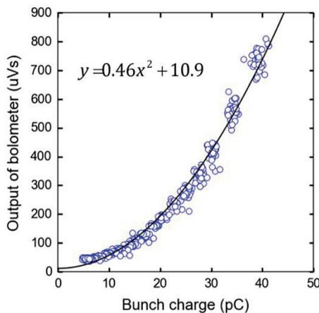
Figure 3: Dependence of intensity of CTR on bunch charge and fitting curve of quadratic function.
