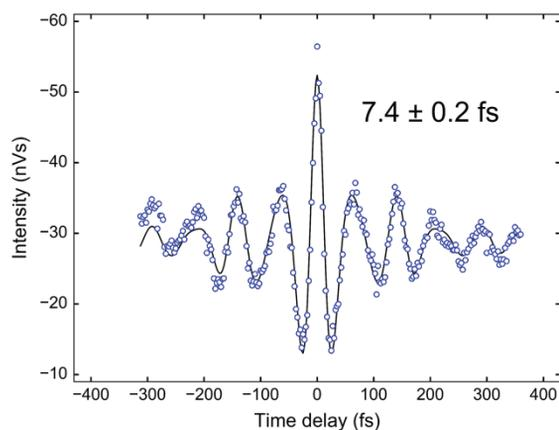
Figure 4: Interferogram of CTR and fitting curve based on sensitivity model.
