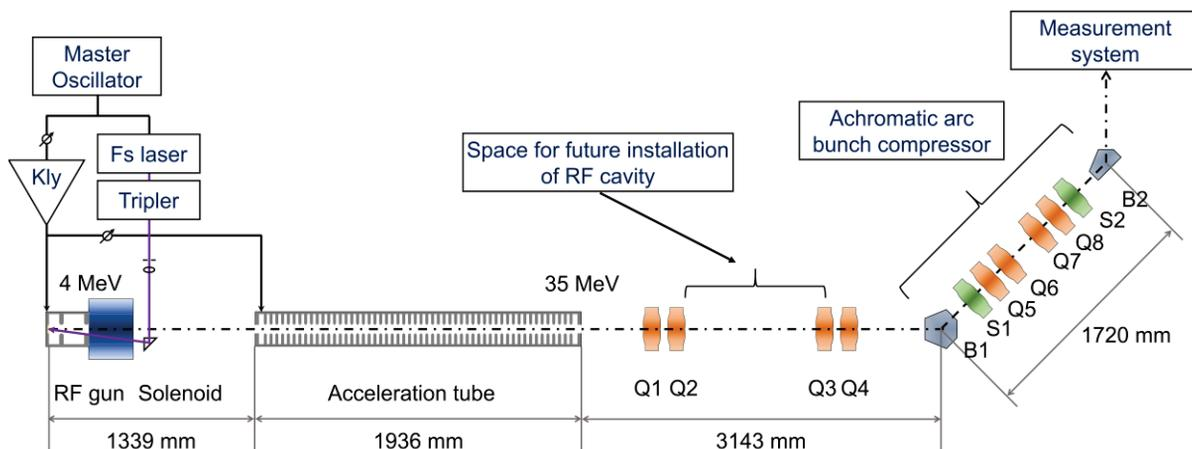
Figure 1: Schematic diagram of a laser photocathode RF electron gun linac and a magnetic bunch compressor. Q: quadrupole magnet; B: bending magnet; S: sextupole magnet.
