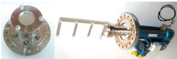
Figure 2: Photos of X-ray detector (left) and mechanical system for wire insertion (right) of BEM.
