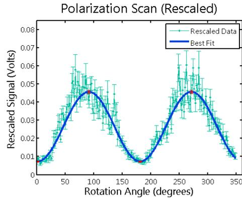
Figure 7: The rescaled data for a 360° rotation of the detector and polarizer ( Fig. 3). The mode used for the fit is Eq. 6. The goodness of fit parameter is  $R^2 = 0.917$ .
