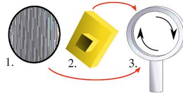
Figure 3: Diagram of Experimental Setup. 1. Wire Polarizer, 2. Detector, 3. Rotating Stand. Red arrows indicate that both the detector and the polarizer are bolted to the rotating stand.
