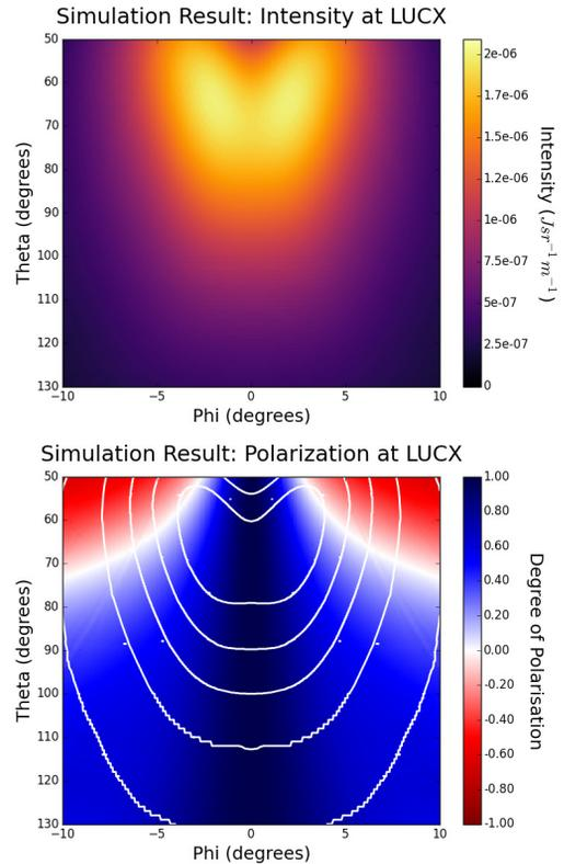
Figure 1: Simulation of intensity (top) and degree of polarization (bottom, contours show intensity), of cSPr generated by the interaction of a 1 mm period grating and an 8 MeV beam.  $\theta$  and  $\phi$  are the angles along and around the beam.
