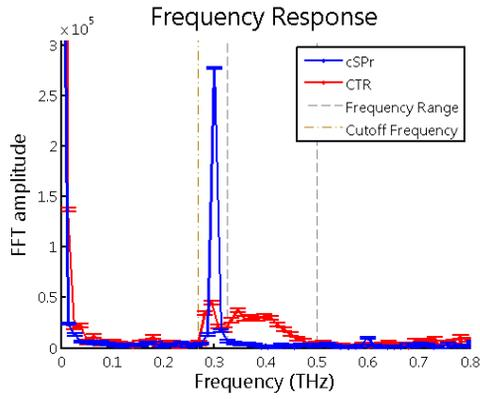
Figure 4: Frequency spectrum of cSPr compared with broadband CTR with the same detector and experimental set-up.
