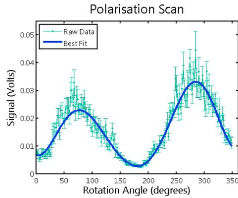
Figure 5: Measured raw data for a 360° rotation of the detector and polarizer (Fig.3). The model used for the fit is Eq. 5 and the goodness of fit parameter is  $R^2 = 0.936$ .
