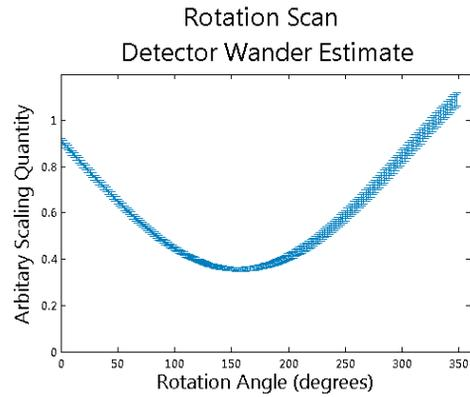
Figure 6: The estimated variation in the signal due to the movement of the detector around the focus of the radiation.
