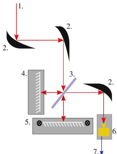
Figure 2: Diagram of Experimental Setup. 1. Radiation from THz Chamber, 2. Parabolic Mirror, 3. Beam Splitter, 4. Plane Mirror, 5. Plane Mirror on Motorised Stand, 6. Detector Mounted on Stand, 7. Signal to ADC or Oscilloscope.
