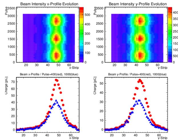
Figure 5: Example of beam transverse profile as recorded by the dose delivery prototype chamber. Top:  $x$  and  $y$  profiles versus beam pulses; bottom:  $x$  and  $y$  profiles corresponding to the highest and lowest intensity pulses. Beam frequency of 10 Hz. The beam oscillations of  $\sim 2$  min period were caused by small uncompensated temperature fluctuations in the cavities.
