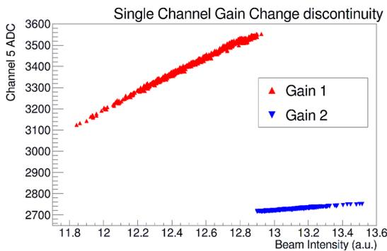
Figure 4: Collected charge (as ADC raw values) on a channel that undergoes gain changes due to the beam intensity pulse-to-pulse variations. Each point represents a pulse. The gap between the two lines of points at the discontinuity ( $x$  12.9) is related to the pedestal of the two gain states as discussed in the text. The slopes of the lines are proportional to the feedback capacitances (referring to Fig. 2:  $C_1 = 10$  pF and  $C_2 = 100$  pF).
