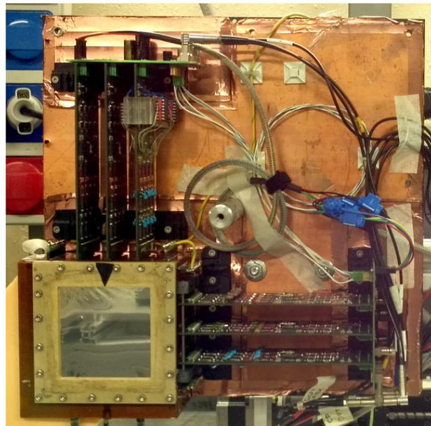
Figure 3: The small chamber prototype (bottom left) and the acquisition electronics, normally shielded by a plastic box with an internal copper layer all around, as visible behind the boards.
