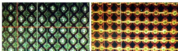
Figure 1: Detail of the layout of the cathode plane with the pad pattern; left: side exposed to the charge collection, right: external side with strips connected to the pads of the other side by filled vias.
