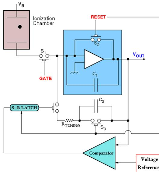
Figure 2: Schematic representation of the adaptive multi gain amplification logic.
