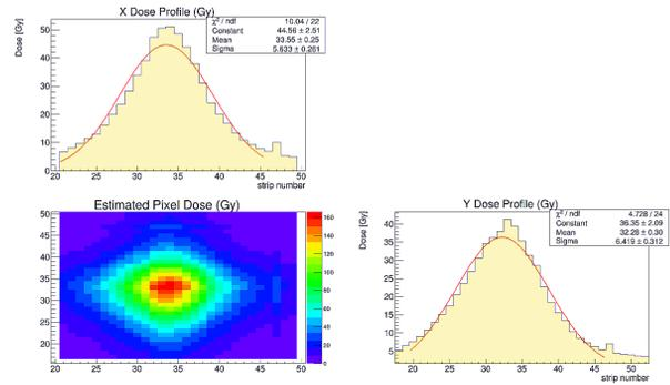
Figure 7: Beam 1-dimensional measured profiles and derived (under specific assumptions of the shape of the beam) 2-dimensional intensity cross section. The red curves are Gaussian fits of the beam profiles.
