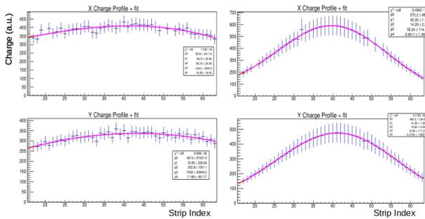
Figure 6: Equalization of the channel responses; left: profiles of the reference run used for the equalization (high voltage is 400 V); right: equalized channel responses (high voltage is 300 V, different position relative to the beam pipe exit window); the error bars represent the statistical errors and are mainly due to the beam fluctuation. The curves on top of the data are Gaussian fits. Three known faulty channels are masked in the  $x$  axis profiles.)
