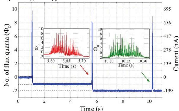
Figure 4: Flux jump of the SQUID signal observed during slow extraction of 5×10<sup>9</sup> Ni<sup>26+</sup> with 125 ms extraction time, i.e. an average current of 60 nA (see text).
