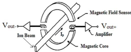
Figure 1: Schematic layout of the novel DCCT.
