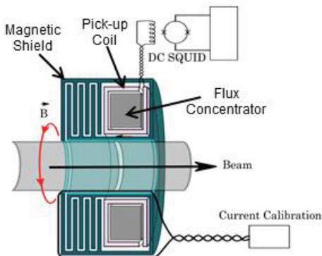
Figure 3: Schematic view of the CCC sensor assembly.
