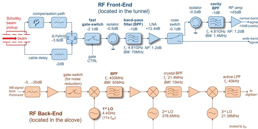
Figure 6: Simplified block schematics of the RF Schottky signal processing.
