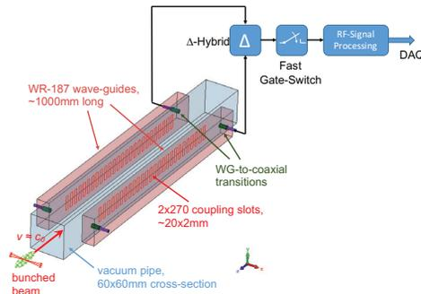
Figure 2: Simplified overview of the LHC *Schottky* monitor system (beam pickup not to scale).
