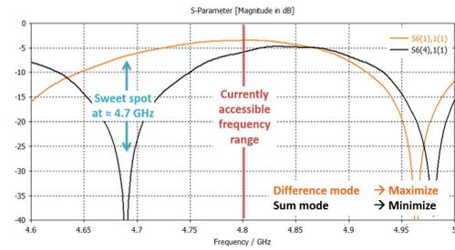
Figure 4: Simulation of the *Schottky* pickup transfer response.
