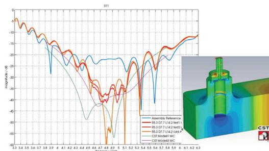
Figure 3: Return-loss of the optimized waveguide-to-coaxial mode launcher.
