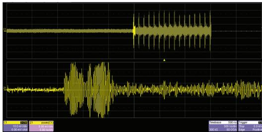
Figure 7: Bunched beam Schottky signals (time domain).
