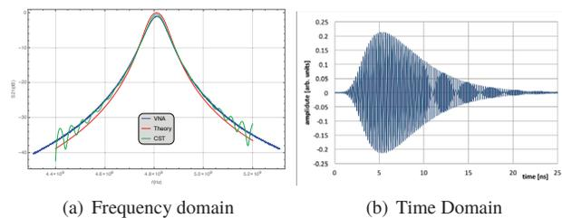
Figure 8: Characteristics of the Bessel interdigital band-pass.
