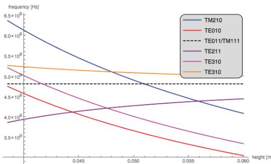
Figure 9: Mode-chart of an ideal “pill-box” resonator.
