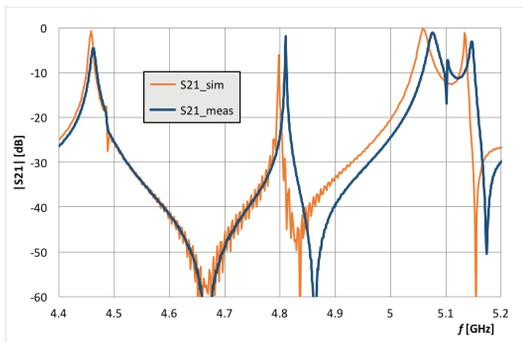
Figure 10:  $|S_{21}(f)|$  transfer function of the cavity band-pass.
