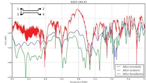
Figure 5: Remaining isolation between the output ports before and after installation of the *Schottky* beam pickup.
