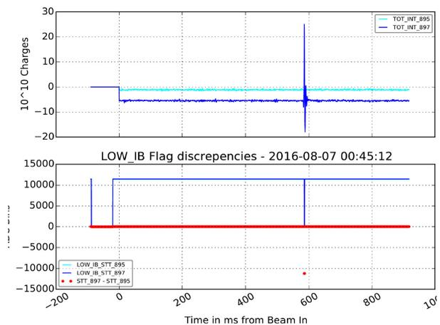
Figure 3: Top Plot : Signal proportional to DC beam current during an SPS Cycle (one trace for each DCCT). Bottom plot : Shows the evolution of the 2 status flags during the cycle (high level = OK for extraction, low level = NOT OK for extraction) and in red, the difference of the two flags.
