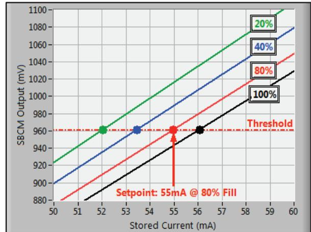
Figure 11: Determining Threshold for SBCM.
