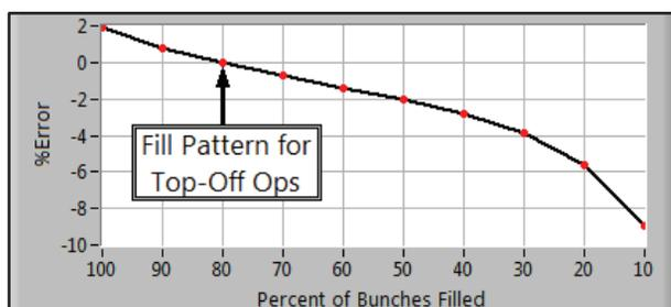
Figure 12: SBCM Error versus Fill Pattern.
