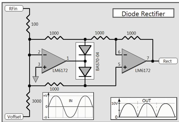
Figure 8: Diode Rectifier Schematic.
