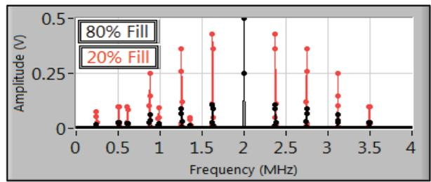
Figure 9: Sideband Dependency on Fill Pattern.
