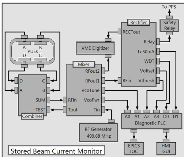
Figure 4: SBCM Block Diagram.
