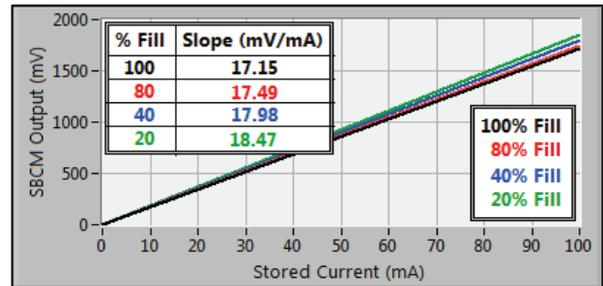
Figure 10: Slope Dependency on Fill Pattern.
