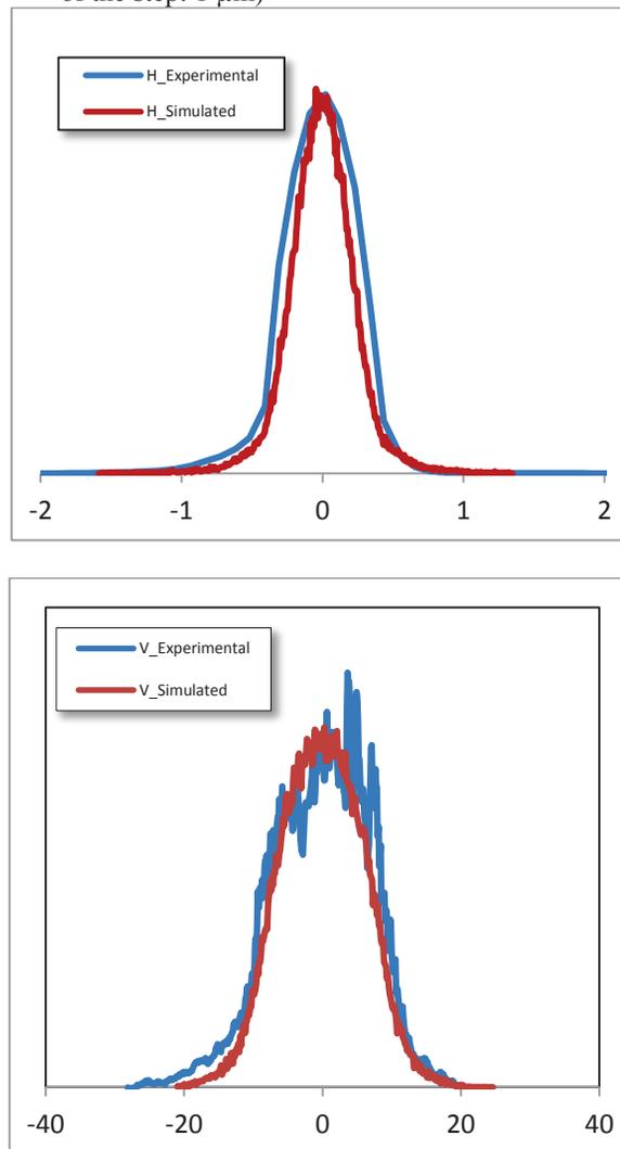
Figure 5: Measurements of the horizontal (up) and vertical (down) transverse beam profiles (mm) with the WS (blue traces) of the accelerated beam (proton 3MeV, 60 mA, pulse duration: 400 $\mu\text{s}$ , repetition: 1s). Red traces are simulated beam profiles.
