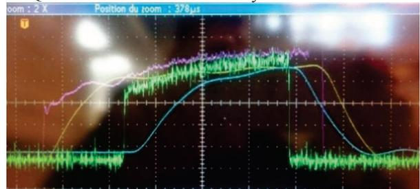
Figure 2: Measurements of the beam current in IPHI. Purple and yellow traces: signals of the ACCT and DCCT upstream the RFQ. Green and blue traces: same measurements with the other couple of ACCT and DCCT downstream the RFQ.
