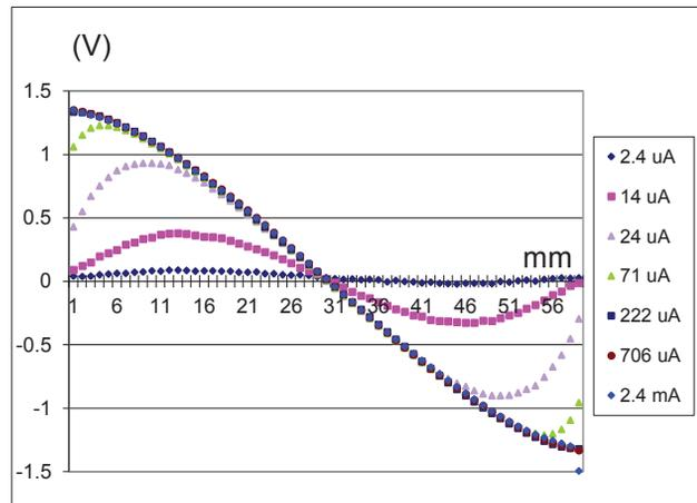
Figure 4: Variation of the output signal of the LR-BPM module with the displacement of the central rod and for different currents in the rod. These measurements have been obtained on our laboratory BPM test bench.
