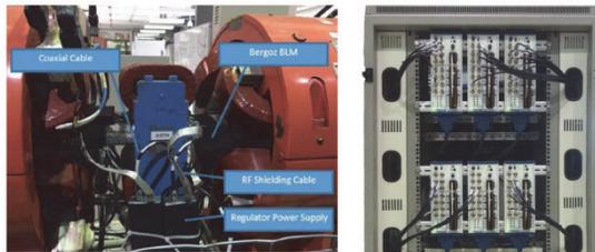
Figure 8: BLM unit (left) and PXIe counter modules (right). [7]
