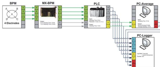
Figure 6: SPS storage ring BPM system. [5]
