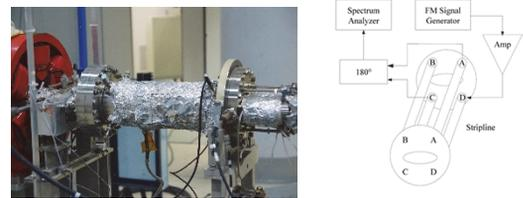
Figure 10: Stripline kicker (right) and real-time tune measurement setup (left) for the SPS storage ring. [3]
