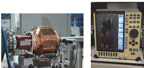
Figure 4: Booster DCCT (left) and oscilloscope displaying beam current in the control room (right).
