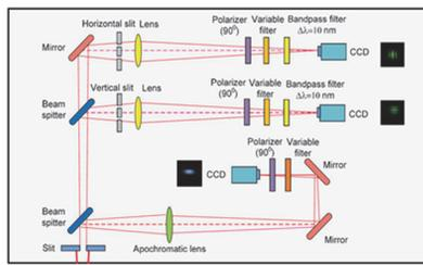
Figure 7: Schematic layout of the transverse beam profile monitor. [6]
