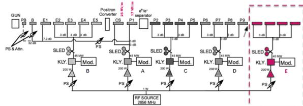
Figure 4: Proposed layout of the RF distribution for the upgraded LINAC.
