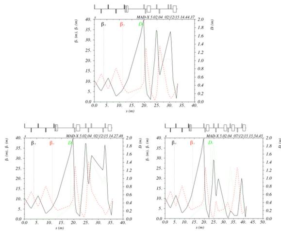
Figure 6: MAD-X results for the  $\beta$  function and dispersion of the present BTF (top) and for the new lines “1” and “2” (bottom left and right respectively).
