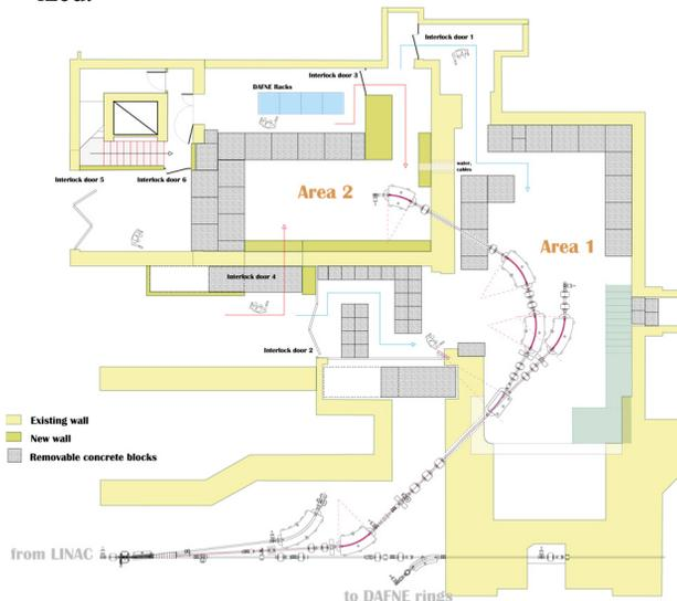
Figure 5: The new BTF lines and the modified layout of the building for hosting two separated experimental areas.
