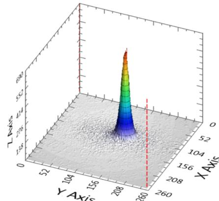
Figure 2: Typical 450 MeV electron beam imaged with the FitPIX detector (1 pixel=55  $\mu\text{m}$ ).
