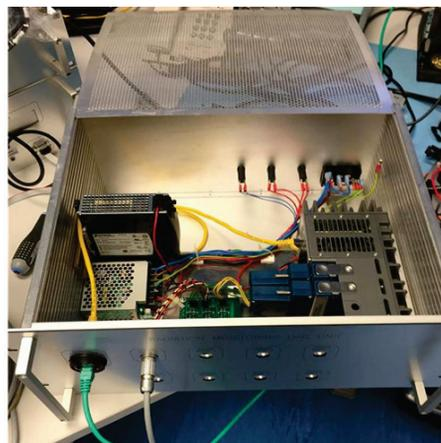
Figure 7: National Instruments cRIO measurement system in custom Schroff chassis.
