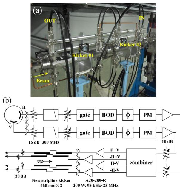
Figure 5: (a) Photo of the installed kicker ducts and (b) block diagram of the PF-AR feedback damper system. PM in the block diagram stands for pulse modulator.
