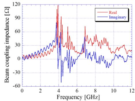
Figure 3: Real and imaginary parts of the longitudinal beam coupling impedance for the improved kicker. The simulated beam bunch length is 8.3 mm (28 ps).
