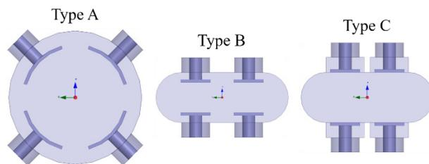
Figure 2: Basic structures considered for the new stripline kicker.
