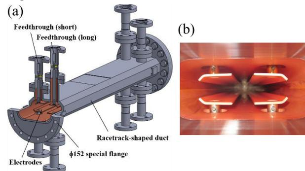
Figure 4: (a) Schematic drawing of the new stripline kicker duct and (b) photo of the inner electrodes.
