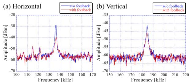
Figure 6: Tune spectra for the (a) horizontal and (b) vertical directions excited by the tune measurement system. The origins of a few peaks on the lower-frequency side of the horizontal tune are unknown.
